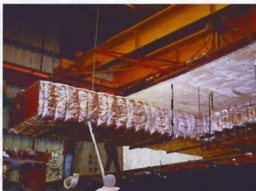
ISO 6944 Ventilation Duct Test
