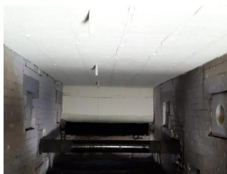
Photo-5 Completed lining after operation
