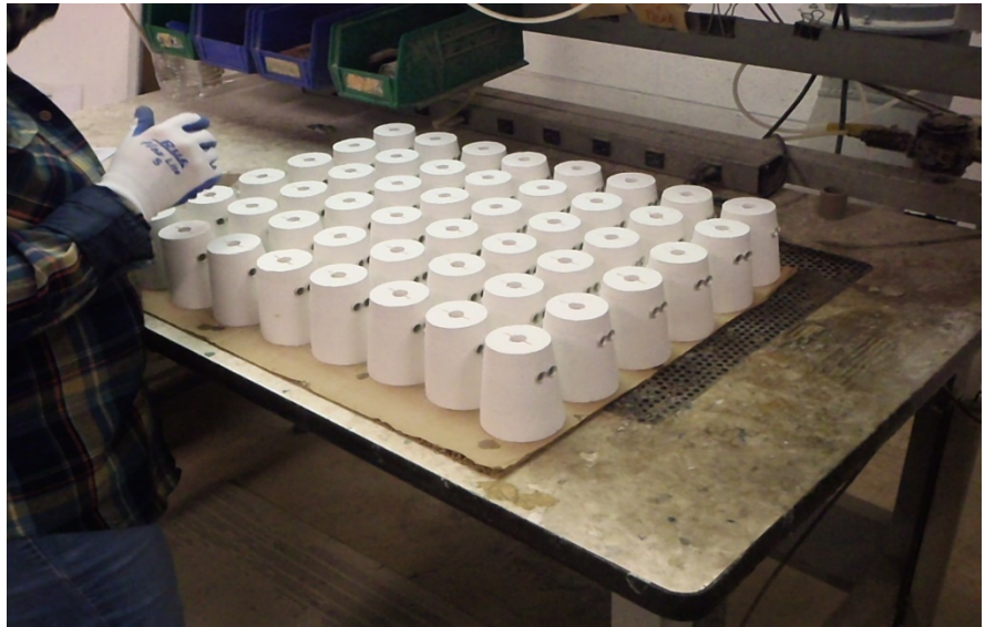
Photo-2 Thermfrax thermic welding crucibles are designed for a variety of ground cable sizes and terminal locations.
