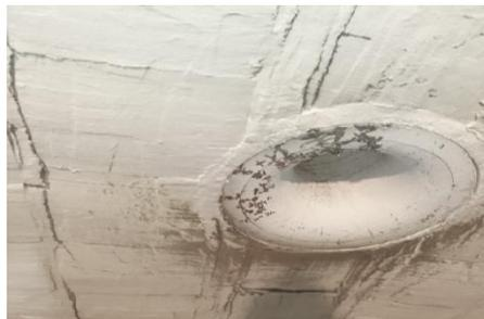
Photo-4 Lining after firing
