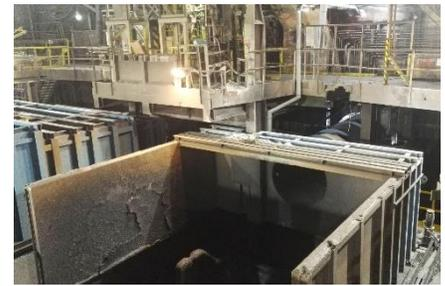
*Photo-4 Metallic deposits peeling away from Silplate Mass 1500*
